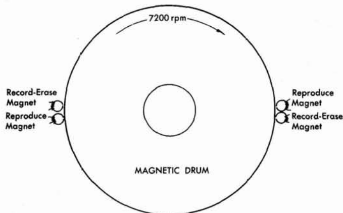
Figure 103. Magnetic Drum Storage Principle
